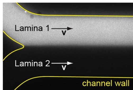
**Figure 1.** Two streams, one containing fluorescent beads, meet but continue as if still confined by channel walls. These non-mixing streams are referred to as lamina and such flow is called laminar flow.
