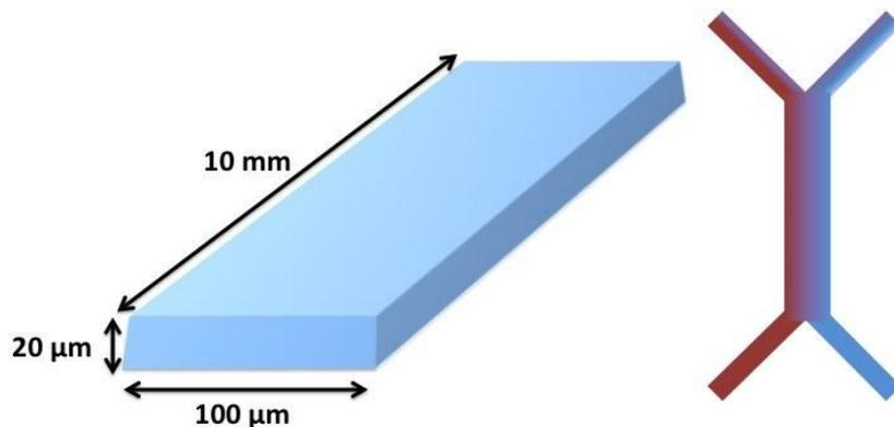
*Figure 3. The dimensions of the H-filter. Right: height, length and width of the main transport channel. Left: example sketch of h-filter device model.*
