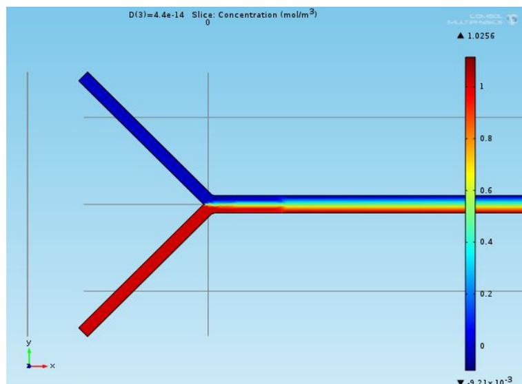
**Figure 4.** Example model of how particles diffuse between flow streams in the H-filter. Red is a concentration of 1 molar and blue is a concentration of 0. The software simulates the effects of diffusion, which can be seen as the mixing of the two colors in the center.
