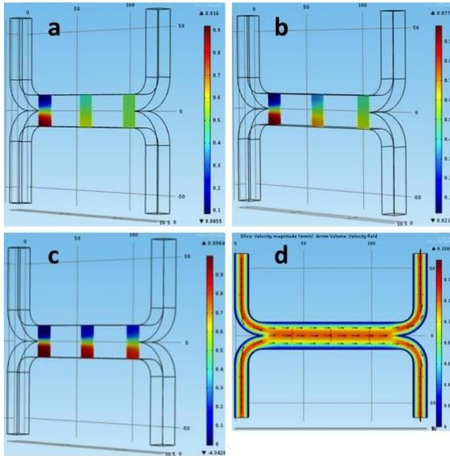
**Figure 5.** (a-c) Example model of how particles of different size, and therefore different diffusion coefficients, diffuse between flow streams in the H-filter. Red is the highest concentration (near  $c_0$  or  $1M$ ), while blue is the lowest (near zero). (d) Velocity profile ( $z$ -plane) of H-filter with particles of one size. Red indicates areas of highest velocity, while blue indicates regions of lowest velocity. Arrows indicate weighted velocity in the device.
