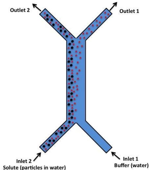
*Figure 2. Small particles (red) diffuse into the diluent stream due to their large diffusion coefficient whereas larger particles (black) don't diffuse as far and remain in the sample stream.*
