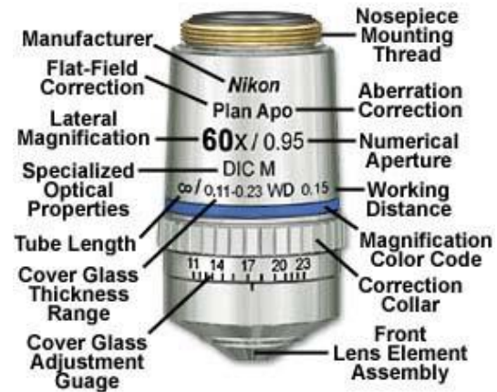
Figure 7. An image of a 60x Plan Apochromat objective with specifications.
